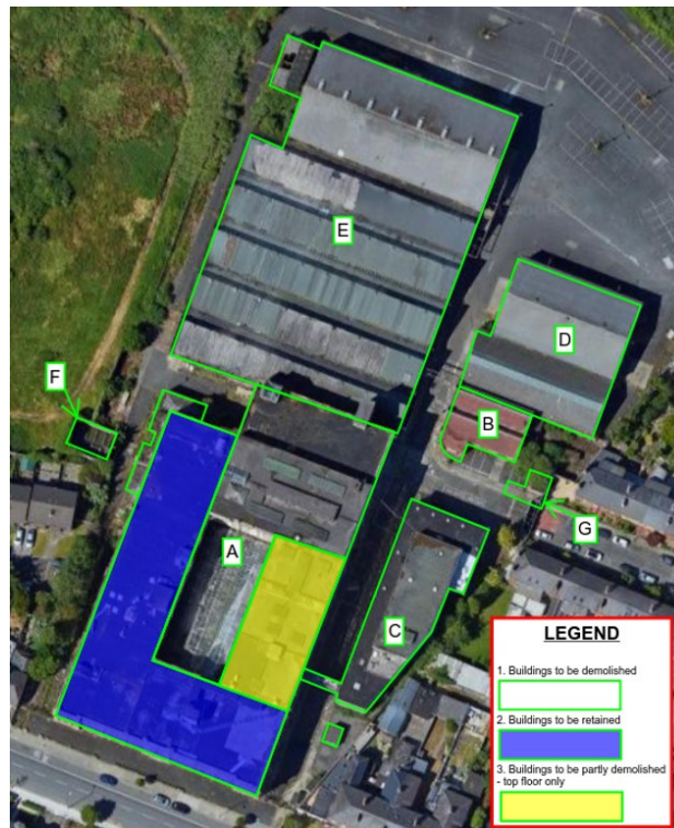
Figure 5: Aerial view of Site Showing Buildings to be Retained, Demolished & Building Footprints. (CDWMP-BMCE)
